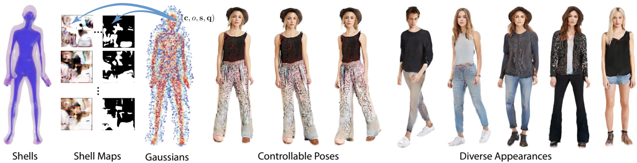
Figure 1. Gaussian Shell Maps. Gaussian Shell Maps is an efficient framework for 3D human generation connecting 3D Gaussians with CNN-based generators. 3D Gaussians are anchored to “shells” derived from the SMPL template [36] (only two shells are visualized for clarity), and the appearance is modeled in texture space. Trained only on 2D images, we show that our method can generate diverse articulable humans in real-time with state-of-the-art quality directly in high resolution without the need for upsampling and hence avoiding aliasing artifacts.
